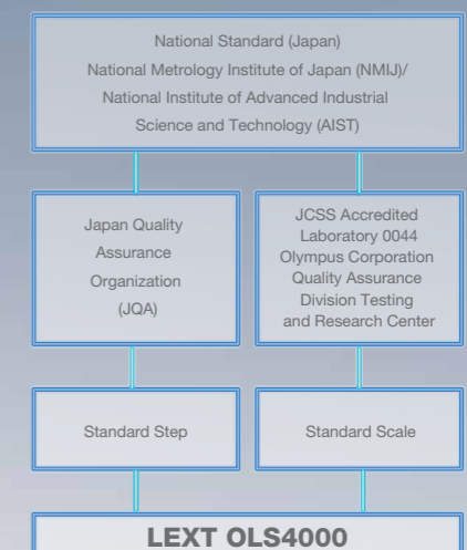
LEXT OLS4000 Traceability System Diagram
