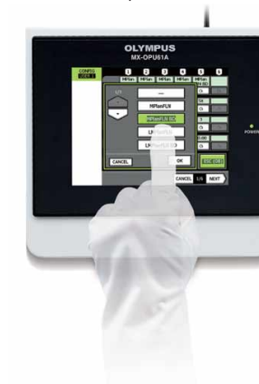
The on-screen buttons accept operations of hand in glove (MX-OPU61A)
