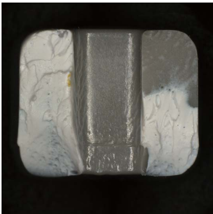
Fractured resin surface
